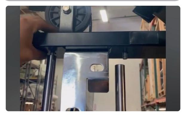
STEP 7. INSTALL THE WEIGHT SELECTOR PIN AND REATTACH CABLE TO THE TOP PLATE AND THEN STORE WEIGHT ADAPTERS ON THE CHROME BRACKET AT THE TOP SO THAT THE CABLE CAN BE TIGHTENED AND ADJUSTED
